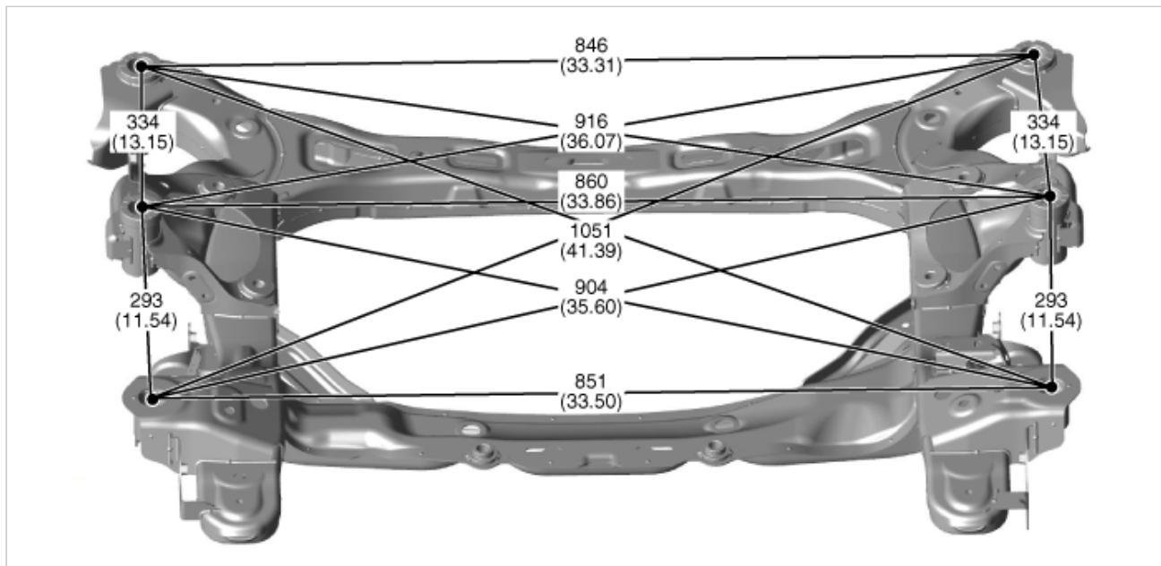
\* These dimensions indicated in this figure are actual-measurement dimensions. [ Unit : mm (inch) ]
