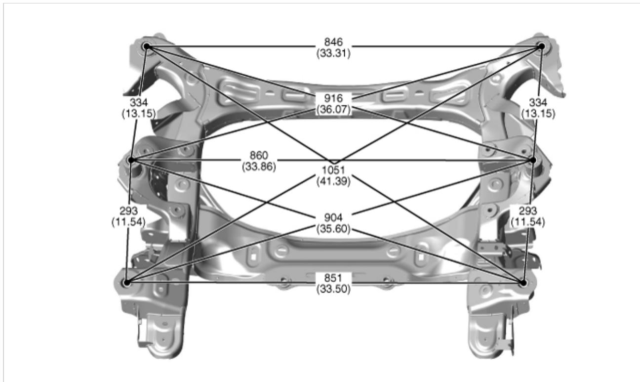
\* These dimensions indicated in this figure are actual-measurement dimensions. [ Unit : mm (inch) ]
