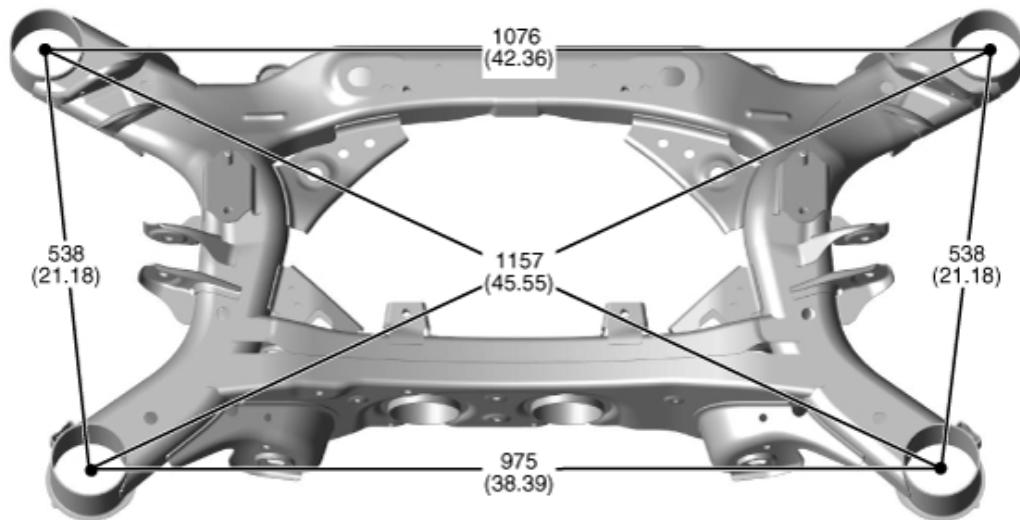
\* These dimensions indicated in this figure are actual-measurement dimensions. [ Unit : mm (inch) ]
